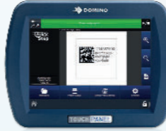
Easy to operate D-Series i-Tech uses QuickStep , our unique simplified operator user interface for effortless control and status reporting. No complex menus or parameters, just enter the job and away you go. • Large user friendly icons and customisable home screen for quick access • Intuitive 3-tiers menu structure makes QuickStep WYSIWYG message creation and editing quick and easy to learn
