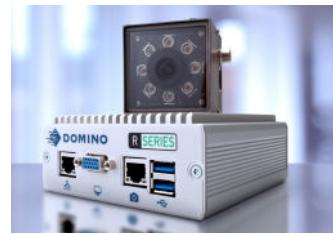
Ensure every code that leaves your factory is present and correct, and free up operator time. With the R-Series, Domino's range of vision control systems, you can automate your code inspection to validate code presence, placement, and readability.
